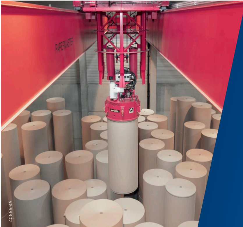
Three Demag overhead travelling cranes with vacuum lifting devices ensure safe roll transport throughout the store
