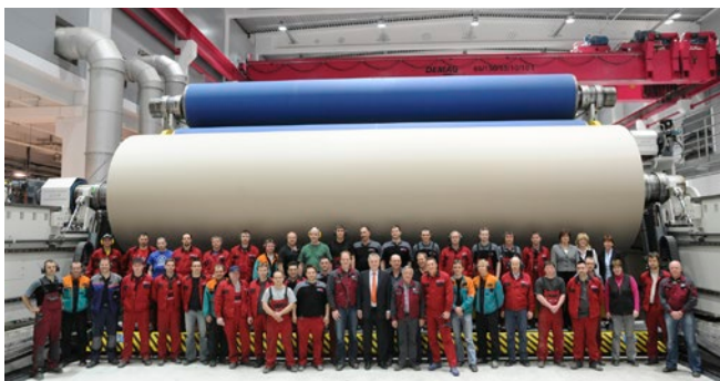
1,800 m/min at a width of 10.20 m: paper machine PM2 operates at world-record speed
