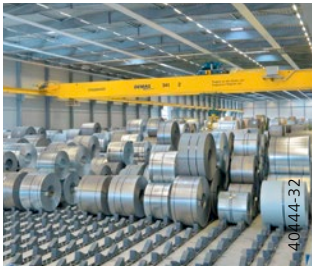
Fully automated coil store with magnets at Becker Stahlservice in Bönen, Germany
