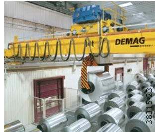
Automatic handling of aluminium coils at Pechiney Rhenalu in Rugles, France
