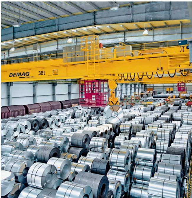
Three Demag Process Cranes fitted with coil magnets on one crane runway
