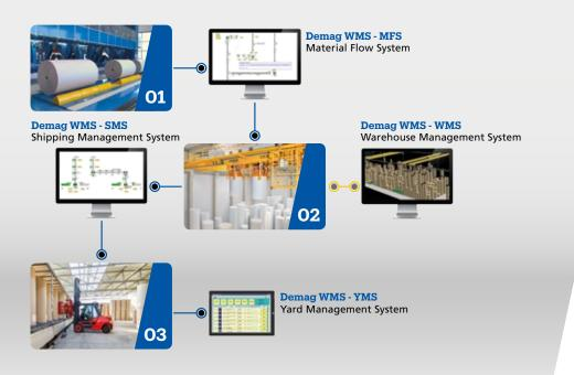
Demag WMS controls all processes: from production planning, warehouse management and shipping management to transport system control
