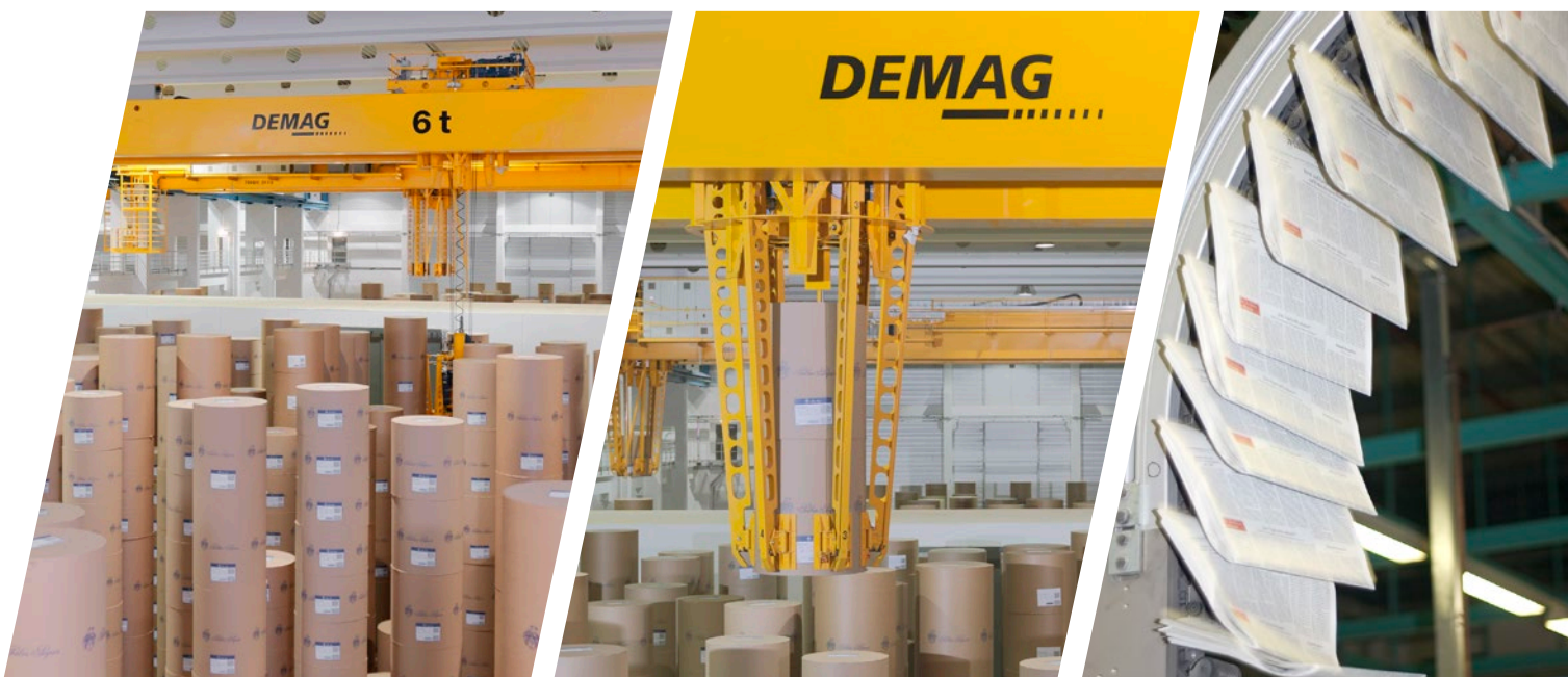
Mechanical grippers set new standards for automated handing of paper rolls
